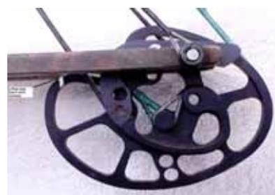
**Safety Note: The only safe way to adjust a braced compound is to use a Bow Press to load the Limbs and remove the tension on the strings and cables. The club has several Bow Presses including several Portable Bow Presses. Members are happy to help you adjust your bow—all you need to do is ask.**
